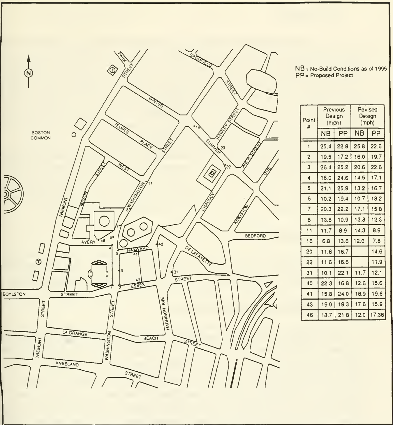
FIGURE V-8 SENSOR LOCATIONS WITH 1% MEAN VELOCITY VALUES
